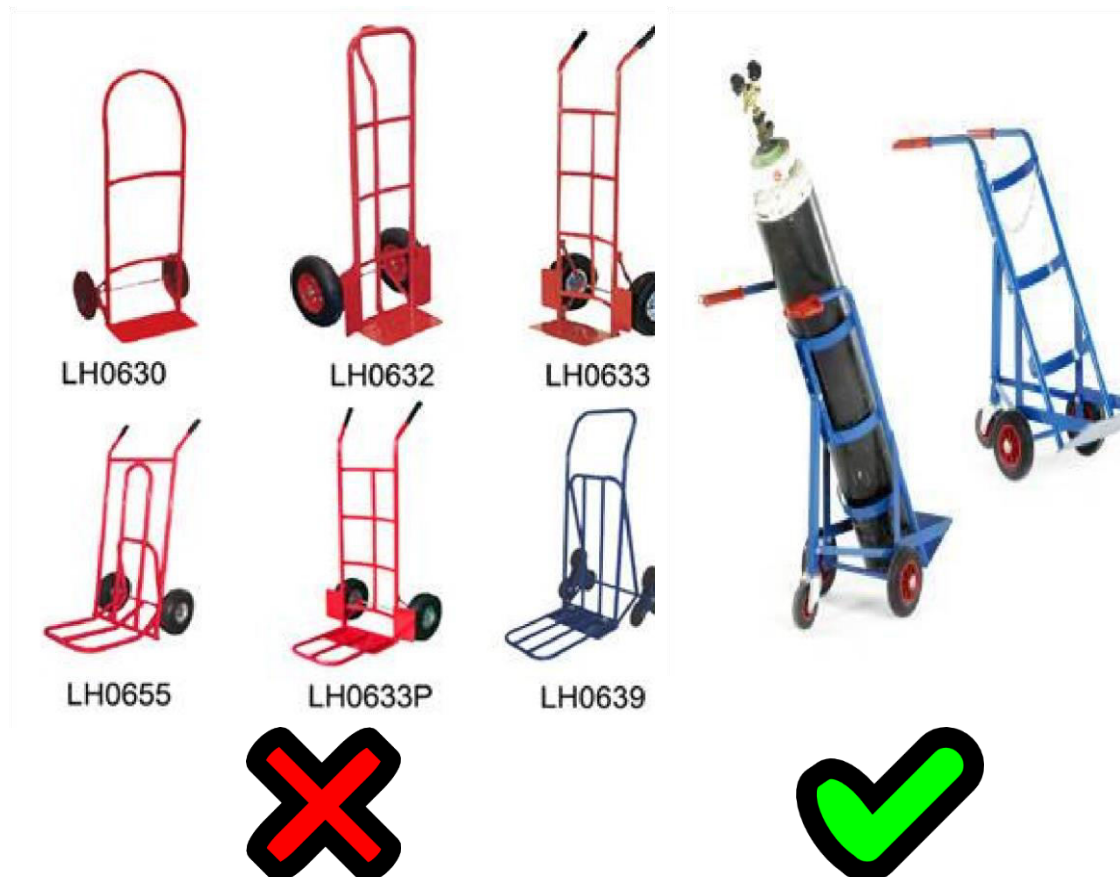
Fig. 5. Trolleys suitable and not for transporting gas cylinders.
