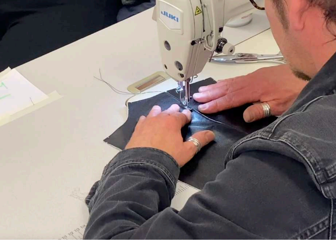
Paul Seville demonstrating machine sewing seamlines on leather.
