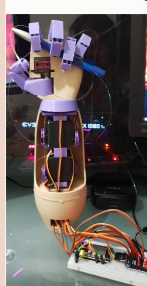
comprised of MG996R metalgeared servos for the fingers, thumb, and forearm. MG90S microservo for the movement of the opposable thumb. ESP32 microcontroller to process, encrypt and send over the built-in WiFi. PCA9685 servo driver that allows I2C communications to all servos
