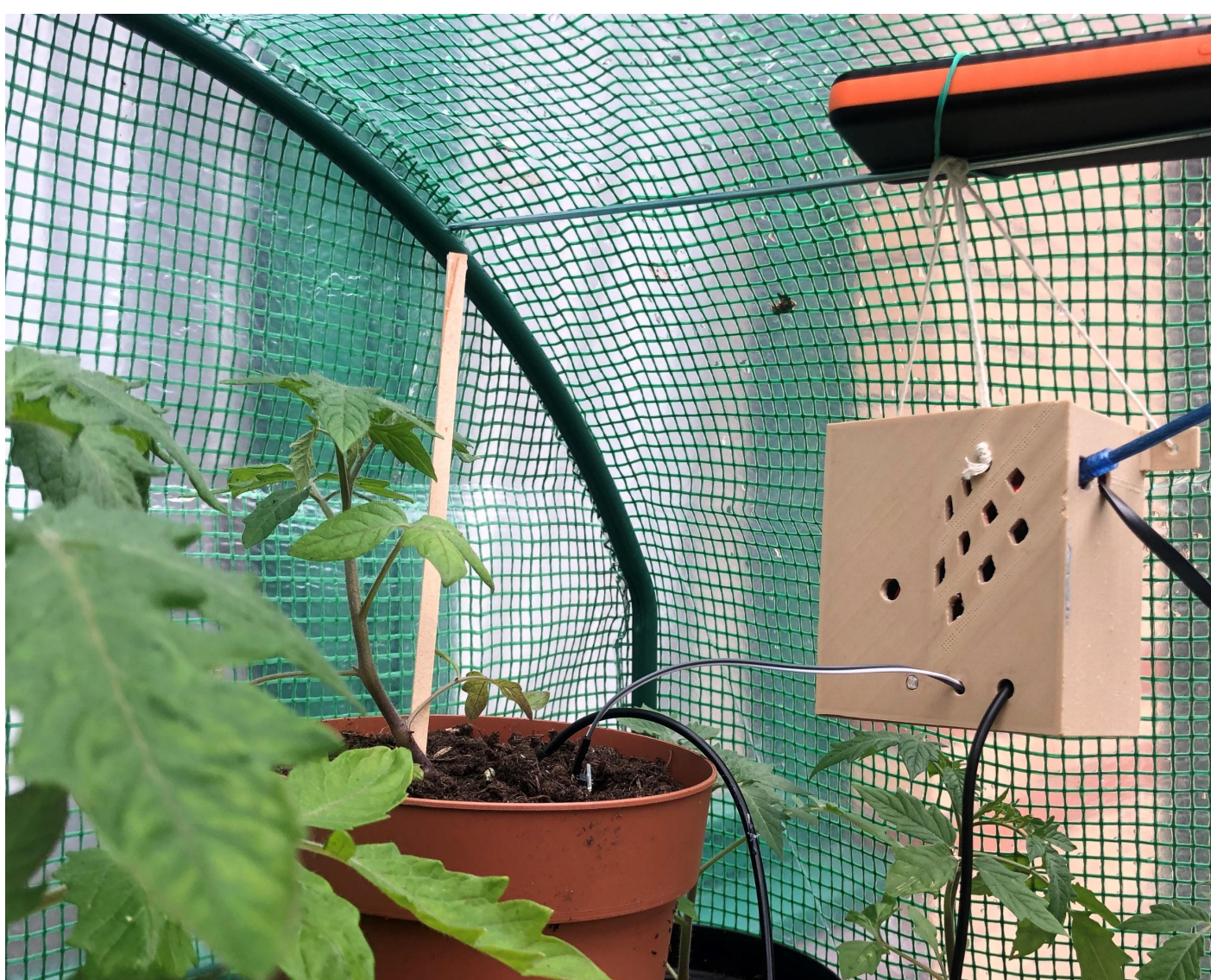
RAHMS Client enclosed in the 3D printed case in the greenhouse with tomato plants.
